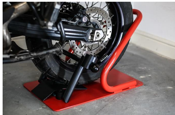
Line up the pin, slide it through, and push the lock down to secure
